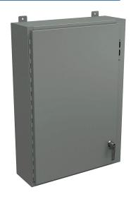
Wiegmann disconnect enclosure, NEMA 12/13, right flange, 36 x 25 x 8in (HxWxD), wall mount, carbon steel, ANSI 61 gray, powder coat finish, single-door, 2-point padlocking handle, purchase subpanel separately.
