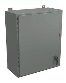
Wiegmann disconnect enclosure, NEMA 12/13, right flange, 30 x 25 x 12in (HxWxD), wall mount, carbon steel, ANSI 61 gray, powder coat finish, single-door, 2-point padlocking handle, purchase subpanel separately.
