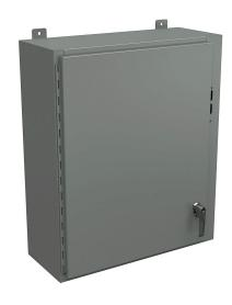
Wiegmann disconnect enclosure, NEMA 12/13, right flange, 30 x  $25 \times 10$  in (HxWxD), wall mount, carbon steel, ANSI 61 gray, powder coat finish, single-door, 2-point padlocking handle, purchase subpanel separately.
