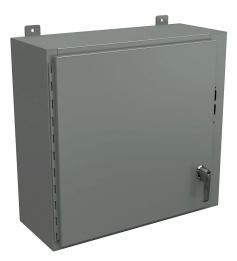
Wiegmann disconnect enclosure, NEMA 12/13, right flange, 24 x 25 x 10in (HxWxD), wall mount, carbon steel, ANSI 61 gray, powder coat finish, single-door, 2-point padlocking handle, purchase subpanel separately.
