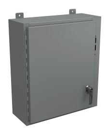
Wiegmann disconnect enclosure, NEMA 12/13, right flange, 24 x 21 x 8in (HxWxD), wall mount, carbon steel, ANSI 61 gray, powder coat finish, single-door, 2-point padlocking handle, purchase subpanel separately.
