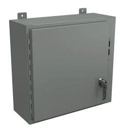
Wiegmann disconnect enclosure, NEMA 12/13, right flange, 20 x 21 x 8in (HxWxD), wall mount, carbon steel, ANSI 61 gray, powder coat finish, single-door, 2-point padlocking handle, purchase subpanel separately.
