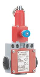
Comepi safety switch, cable-pull interlock, with reset, 15m maximum pull cable length, (1) N.C. safety output(s), (1) N.O. monitoring output(s), zinc alloy body, thermoplastic head, (3) 1/2in NPT cable entries.
