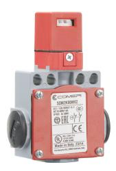
Comepi safety switch, tongue (key) interlock, 360-degree adjustable head, (2) N.C. safety output(s),  $59 \times 100 \times 32$ mm, zinc alloy body, thermoplastic head.
