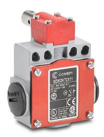
Comepi safety switch, hollow shaft hinge interlock, slow action break before make, (1) N.C. safety output(s), die-cast aluminum body, plastic head, (3) 1/2in NPT cable entries.
