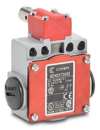
Comepi safety switch, hollow shaft hinge interlock, slow action, (2) N.C. safety output(s), die-cast aluminum body, plastic head, 12mm diameter x 20mm length shaft, (3) 1/2in NPT cable entries.
