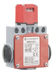
Comepi safety switch, tongue (key) interlock, 90-degree adjustable head, (1) N.C. safety output(s), (1) N.O. monitoring output(s), 59 x 100 x 32mm, zinc alloy body, thermoplastic head.
