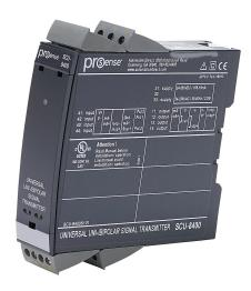
ProSense signal conditioner, isolated, unipolar or bipolar current, voltage input, unipolar or bipolar current, voltage output, 21.6-253 VAC/19.2-300 VDC operating voltage, 35mm DIN rail mount, removable screw terminal plugs.
