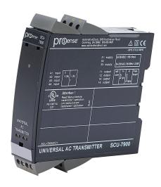
ProSense AC signal conditioner, isolated, AC current, AC voltage input, current or voltage output, 21.6-253 VAC/19.2-300 VDC operating voltage, 35mm DIN rail mount, removable screw terminal plugs.
