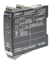
ProSense signal conditioner, isolated, frequency input, current, voltage or frequency output, 21.6-253 VAC/19.2-300 VDC operating voltage, 35mm DIN rail mount, removable screw terminal plugs.
