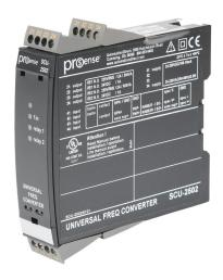
ProSense signal conditioner, isolated, frequency input, relay output, 21.6-253 VAC/19.2-300 VDC operating voltage, 35mm DIN rail mount, removable screw terminal plugs.
