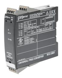
ProSense signal conditioner, isolated, frequency input, current, voltage or relay output, 21.6-253 VAC/19.2-300 VDC operating voltage, 35mm DIN rail mount, removable screw terminal plugs.
