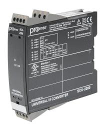
ProSense signal conditioner, isolated, current, voltage, potentiometer, RTD or thermocouple input, deg F or deg C, frequency output, 21.6-253 VAC/19.2-300 VDC operating voltage, 35mm DIN rail mount, removable screw terminal plugs.
