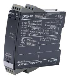
ProSense signal conditioner, isolated, current, voltage, RTD, thermocouple or potentiometer input, deg F or deg C, current, voltage or relay output, 21.6-253 VAC/19.2-300 VDC operating voltage, 35mm DIN rail mount, removable screw terminal plugs.
