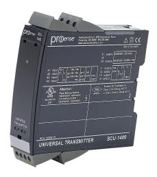
ProSense signal conditioner, isolated, current, voltage, RTD, thermocouple or potentiometer input, deg F or deg C, current or voltage output, 21.6-253 VAC/19.2-300 VDC operating voltage, 35mm DIN rail mount, removable screw terminal plugs.
