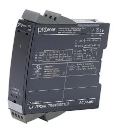
ProSense signal conditioner, isolated, current, voltage, RTD, thermocouple or potentiometer input, deg F or deg C, current or voltage output, 21.6-253 VAC/19.2-300 VDC operating voltage, 35mm DIN rail mount, removable screw terminal plugs.
