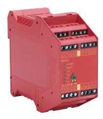
IDEM safety relay, emergency stop and safety gates, 2-channel, 24 VAC/VDC, (7) N.O. safety output(s), (3) N.C. monitoring output(s), fixed screw terminals.
