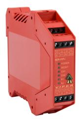
IDEM safety relay, OSSD and light curtain controller, 2-channel, 24 VDC, (3) N.O. safety output(s), (1) N.C. monitoring output(s), fixed screw terminals.
