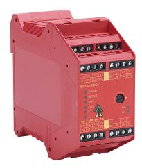
IDEM safety relay, emergency stop and safety gates, release delay, 0 to 30 seconds, 2-channel, 24 VAC/VDC, (4) N.O. time delay and (3) N.O safety output(s), (2) N.C. time delay and (1) N.C monitoring output(s), fixed screw terminals.
