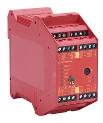
IDEM safety relay, emergency stop and safety gates, release delay, 0 to 30 seconds, 2-channel, 24 VAC/VDC, (4) N.O. time delay and (3) N.O safety output(s), (2) N.C. time delay and (1) N.C monitoring output(s), fixed screw terminals.
