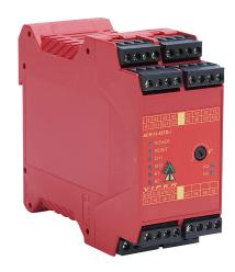
IDEM safety relay, emergency stop and safety gates, release delay, 0 to 30 seconds, 2-channel, 24 VAC/VDC, (4) N.O. time delay and (3) N.O safety output(s), (2) N.C. time delay and (1) N.C monitoring output(s), pluggable screw terminals.
