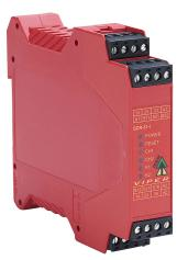
IDEM safety relay, emergency stop and safety gates, 2-channel, 24 VAC/VDC, (3) N.O. safety output(s), (1) N.C. monitoring output(s), pluggable screw terminals.
