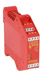
IDEM safety relay, two-hand control, 2-channel, 24 VAC/VDC, (2) N.O. safety output(s), fixed screw terminals.
