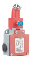
Comepi safety switch, cable-pull interlock, with reset, 25m maximum pull cable length, (2) N.C. safety output(s), (1) N.O. monitoring output(s), die-cast aluminum body, thermoplastic head, (3) 1/2in NPT cable entries.
