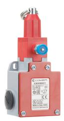
Comepi safety switch, cable-pull interlock, with reset, 25m maximum pull cable length, (1) N.C. safety output(s), (1) N.O. monitoring output(s), die-cast aluminum body, thermoplastic head, (3) 1/2in NPT cable entries.
