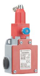
Comepi safety switch, cable-pull interlock, with reset, 25m maximum pull cable length, (3) N.C. safety output(s), die-cast aluminum body, thermoplastic head, (3) 1/2in NPT cable entries.
