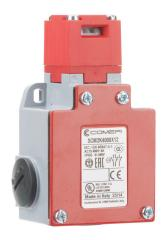
Comepi safety switch, tongue (key) interlock, 90-degree adjustable head, (2) N.C. safety output(s), (1) N.O. monitoring output(s), 62 x 108 x 43mm, die-cast aluminum body, thermoplastic head.
