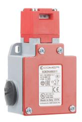
Comepi safety switch, tongue (key) interlock, 90-degree adjustable head, (1) N.C. safety output(s), (1) N.O. monitoring output(s), 62 x 108 x 43mm, die-cast aluminum body, thermoplastic head.
