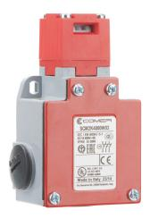
Comepi safety switch, tongue (key) interlock, 90-degree adjustable head, (3) N.C. safety output(s),  $62 \times 108 \times 43$ mm, diecast aluminum body, thermoplastic head.
