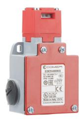
Comepi safety switch, tongue (key) interlock, 90-degree adjustable head, (3) N.C. safety output(s),  $62 \times 108 \times 43$ mm, diecast aluminum body, thermoplastic head.
