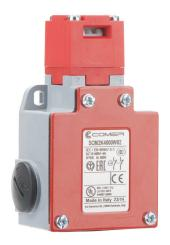
Comepi safety switch, tongue (key) interlock, 90-degree adjustable head, (2) N.C. safety output(s),  $62 \times 108 \times 43$ mm, diecast aluminum body, thermoplastic head.
