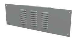
Saginaw skirt kit, 11.94 x 35.75in, carbon steel, ANSI 61 gray, powder coat finish, vented. For use with 36-44in wide floormount enclosures on 12in floor stands.
