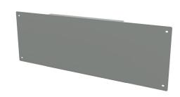
Saginaw skirt kit, 11.94 x 35.75in, carbon steel, ANSI 61 gray, powder coat finish. For use with 36-44in wide floor-mount enclosures on 12in floor stands.
