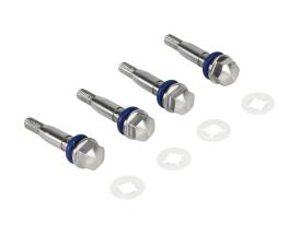
Saginaw sanitary captive screw, replacement, #10-32 UNF x 1.250in, flanged hex head, 316 stainless steel. Package of 4. For use with Saginaw SCE-xxKJxxxxSSST sanitary enclosures. Silicone retainer and blue silicone O-ring included.
