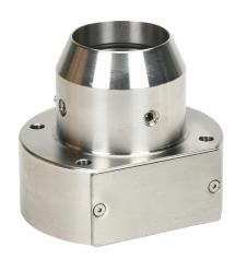
Saginaw suspension arm fitting, floor stand with cable outlet, 304 stainless steel, #4 brush finish. For use with 2.38in round tube suspension arm profile.
