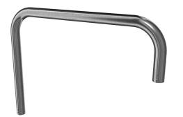
Saginaw suspension arm profile, round S-bend, 2.38in OD, 39.37 x 17.72in offset, 304 stainless steel, #4 brush finish.
