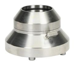
Saginaw suspension arm fitting, swivel coupling, 350 degrees movement range, 304 stainless steel, #4 brush finish. For use with 2.38in round tube suspension arm profile.
