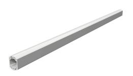
Saginaw suspension arm profile, closed tube, 3.54 x 2.56in, 78.7in length, 6060T66 aluminum.
