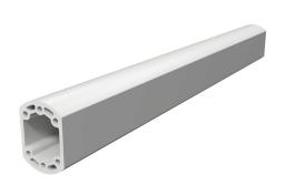
Saginaw suspension arm profile, closed tube, 3.54 x 2.56in, 29.5in length, 6060T66 aluminum.
