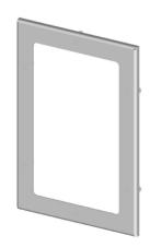
Saginaw enclosure window, 9.25 x 5.75in window, UV-resistant polycarbonate, carbon steel, ANSI 61 gray, powder coat finish, oil-resistant gasket. For use with NEMA 4 enclosures. Mounting hardware included.
