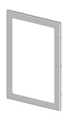
Saginaw enclosure window, 13.25 x 8.25in window, UV-resistant polycarbonate, carbon steel, ANSI 61 gray, powder coat finish, oil-resistant gasket. For use with NEMA 4 enclosures. Mounting hardware included.
