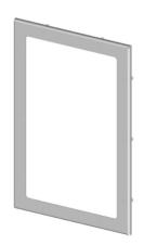
Saginaw enclosure window, 13.25 x 8.25in window, UV-resistant polycarbonate, 304 stainless steel, #4 brush finish, oil-resistant gasket. For use with NEMA 4X enclosures. Mounting hardware included.
