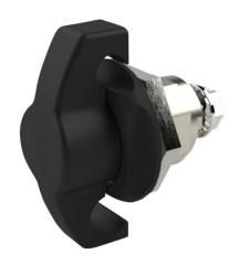
Saginaw enclosure latch, replacement, padlocking, 1/4-turn wing knob, 1-point, die-cast zinc, black matte finish. For use with Enviroline series enclosures. (1) SCE-102804 cam included.
