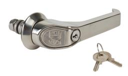
Saginaw latch handle, replacement, 5in, keylocking/padlocking, 1/4-turn, stainless steel. For use with Saginaw enclosures with 3-point door hardware. (2) SCE-KC101 keys included. Requires SCE-ARK36 or SCE-103370 door rod kit or SCE-3PTSMC cam.
