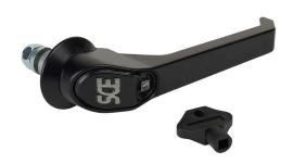
Saginaw latch handle, replacement, 7in, 7mm square, 1/4-turn, die-cast zinc, black matte finish. For use with Saginaw enclosures with 3-point door hardware. (1) SCE-101695 key included. Requires SCE-ARK36 door rod kit or SCE-102237 cam.
