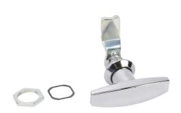
Saginaw enclosure latch, replacement, 1/4-turn tee handle, 1-point, die-cast zinc, chrome finish. For use with Enviroline series enclosures. (1) SCE-102804 cam included.
