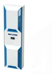
Saginaw NextGen Enviro-Therm air conditioner, 6800 BTU/H, R-134a, 230 VAC operating voltage, carbon steel housing, RAL 7035 light gray, side mount. For use with NEMA/UL Type 3R, 4 & 12 enclosures.
