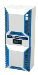
Saginaw NextGen Enviro-Therm air conditioner, 2320 BTU/H, R-134a, 460 VAC operating voltage, carbon steel housing, RAL 7035 light gray, side mount. For use with NEMA/UL Type 3R, 4 & 12 enclosures.
