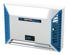
Saginaw NextGen Enviro-Therm air conditioner, 1870 BTU/H, R-134a, 115 VAC operating voltage, carbon steel housing, RAL 7035 light gray, filter-free, side mount. For use with NEMA/UL Type 3R, 4 & 12 enclosures.
